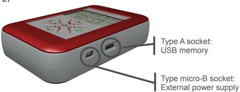
Switch over from internal to external power supply can be done by simply plugging in a USB cable connected to an external power source. This does not cause any operational interruption and is very helpful in case data logging to a USB memory needs to be extended to a much longer time frame, such as for documentation purposes.
